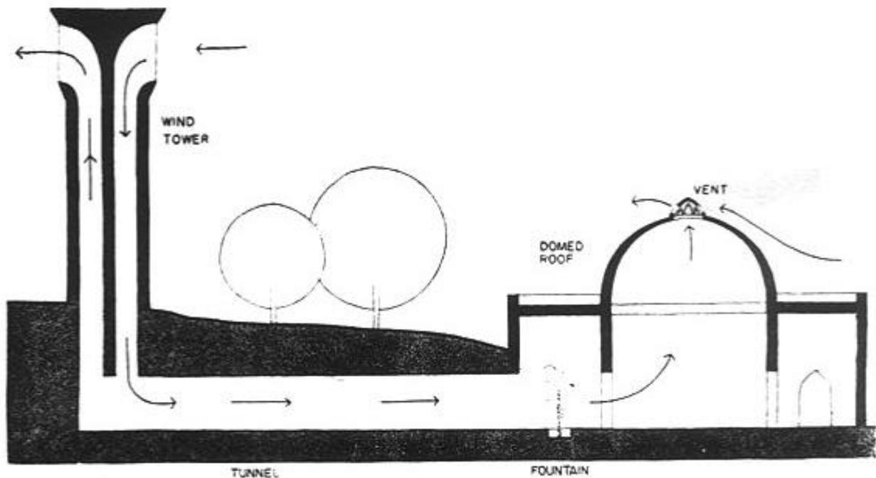
Fig. 13 Iranian cooling system using wind tower, underground funnel evaporative cooling and natural ventilation.
