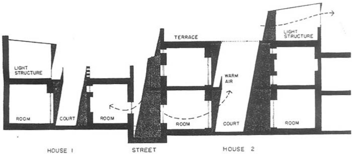
Fig. 16 Typical section through Shahjahanabad houses. The main building is massive while a light-weight structure is built above it
