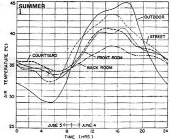
Fig. 15 Measured temperatures and airflow in a house at Jaisalmer. During the calm periods, the courtyard effect brings cool air into the building
