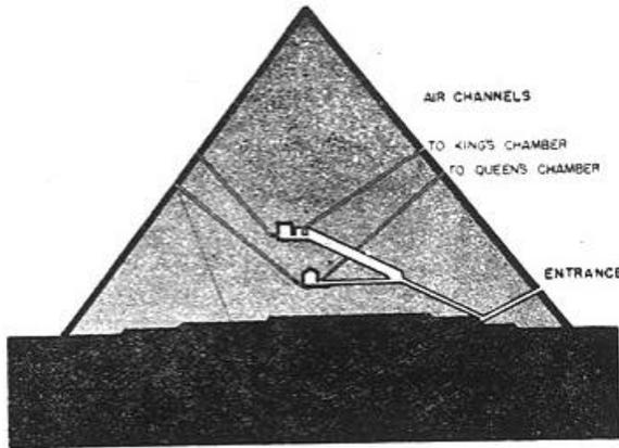
Fig. 17 Section through the pyramid of Cheops at Gizeh. Channels were provided for ventilation with cooled air
