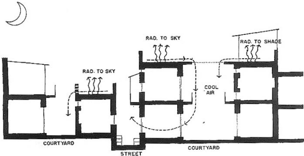
Fig.3 Typical section through Shahjahanabad House. To Facilitate the moment of cool air into the house, parapets are not built towards the courtyard
