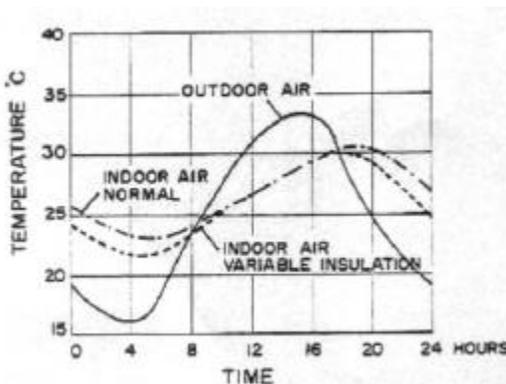
FIG. 11-EFFECT OF VARIABLE INSULATION
