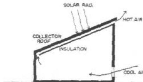
FIG. 12-SOLAR INDUCED VENTILATION
