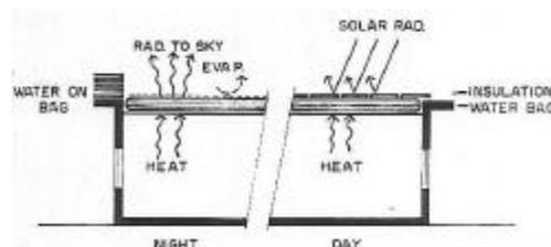
FIG. 17-SKYTHERM COOLING
