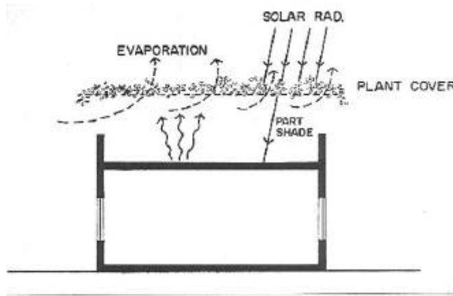
FIG. 5-ROOF SHADING BY VEGETATION
