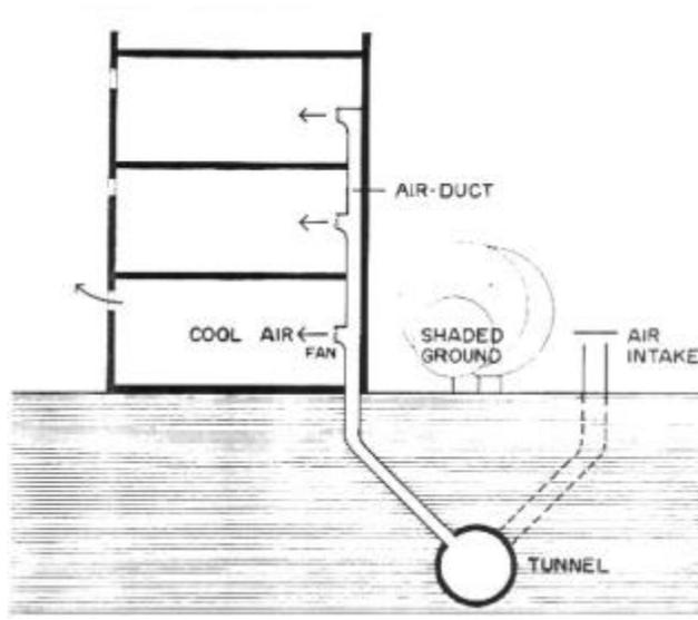
FIG. 13-TUNNEL COOLING
