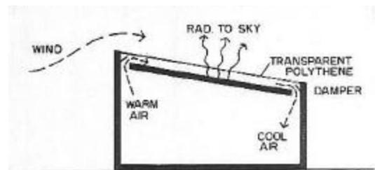
FIG. 15-RADIATIVE COOLING-THERMOSYPHON
