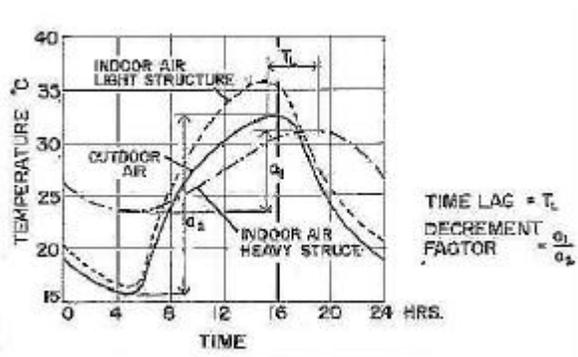
FIG. 8-EFFECT OF THERMAL CAPACITY
