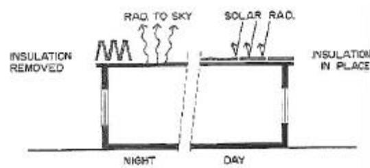
FIG. 10-VARIABLE INSULATION ON ROOF
