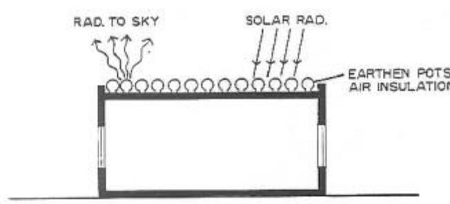
FIG. 6-ROOF SHADING BY POTS
