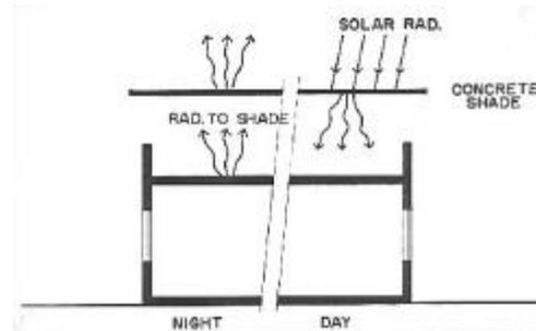
FIG. 4-ROOF SHADING
